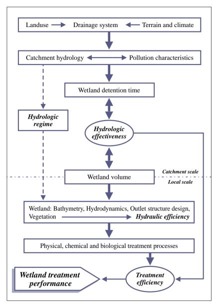
Figure 3: Interaction of wetland design elements
