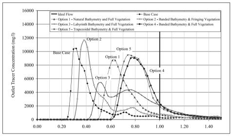
Figure 13: Tracer responses from two-dimensional modelling for five different improvement options for the Monash University Research Wetland
