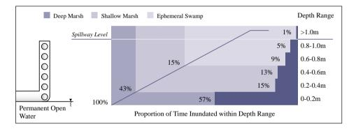
Figure 15: Hydrologic regime for a wetland with a riser outlet
