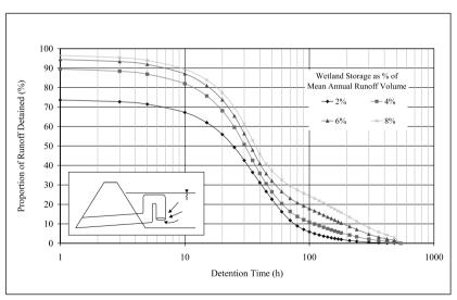
Figure 8: PRTD curves for a culvert outlet
