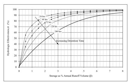
Figure 5: Hydrologic effectiveness curves for wetlands in Melbourne
