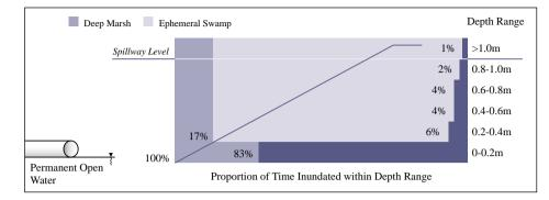
Figure 14: Hydrologic regime for a wetland with a culvert outlet
