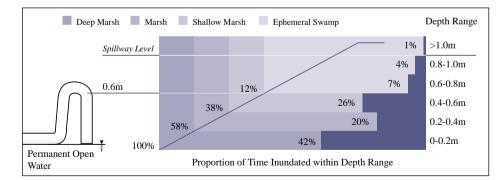
Figure 16: Hydrologic regime for a wetland with a siphon outlet
